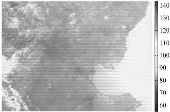
(b) 逐探元定标后图像 (b) Calibrated image detector by detector
